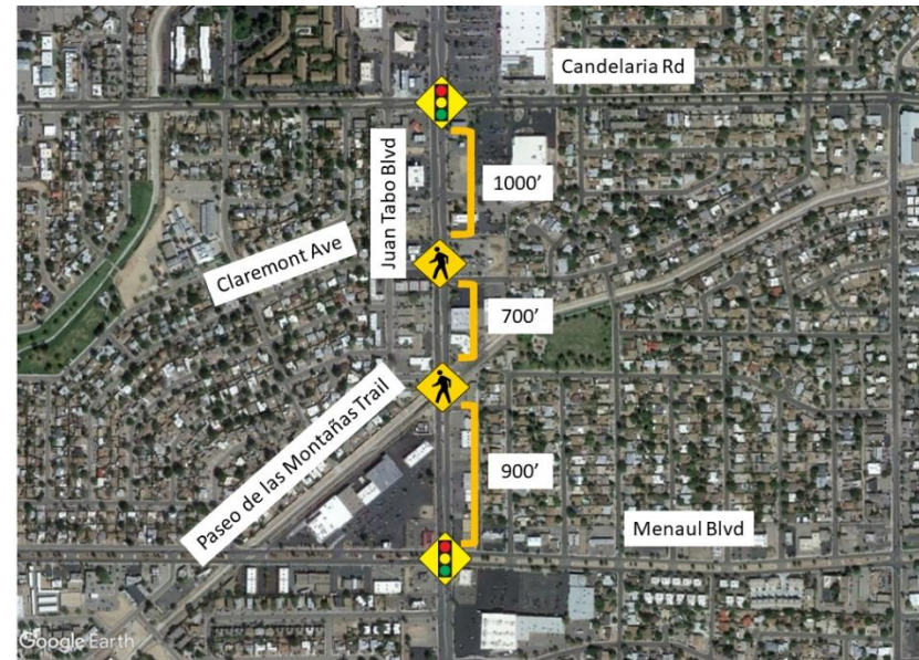
Figure 44: Adjacent Crossing Locations at Juan Tabo Blvd
