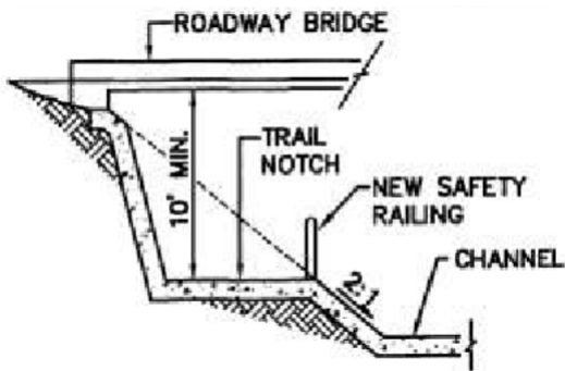
Figure 11: Trail Underpass Notched Into Side of Channel
