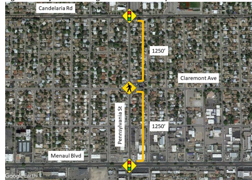
Figure 54: Adjacent Crossing Locations at Pennsylvania St
