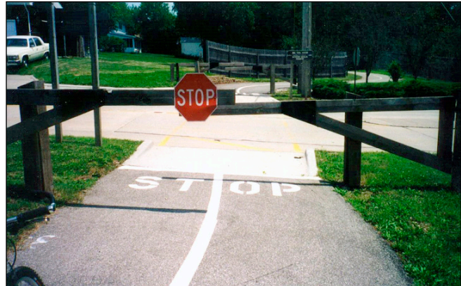
Figure 5-21: Gates across a bicycle path (not recommended)
